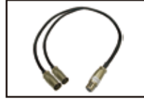
XLR4P-D F P U2 for Digital FPU XLR4P(M) × 2 1:- 4:+ → XLR4P(M) × 2 1,2:- 3,4:+ length : 1m
