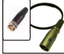
XLR4P-D F P U2 for Digital FPU XLR4P(M) × 2 1:- 4:+ → XLR4P(M) × 2 1,2:- 3,4:+ length : 1m
